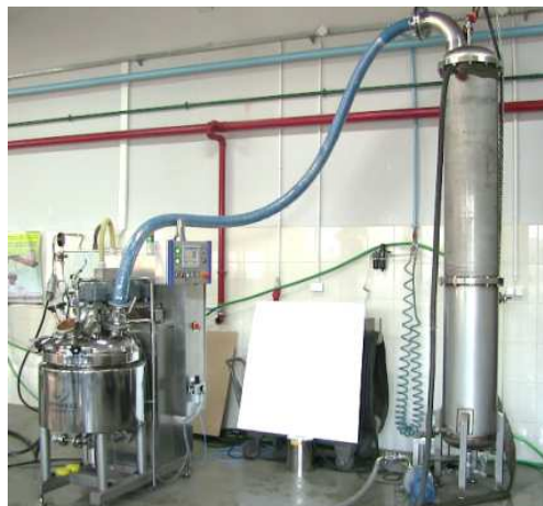
Rysunek 1. Stanowisko badawcze do zagęszczania produktów i poboru skroplin Experimental stand for concentration of products and for sampling of condensates
