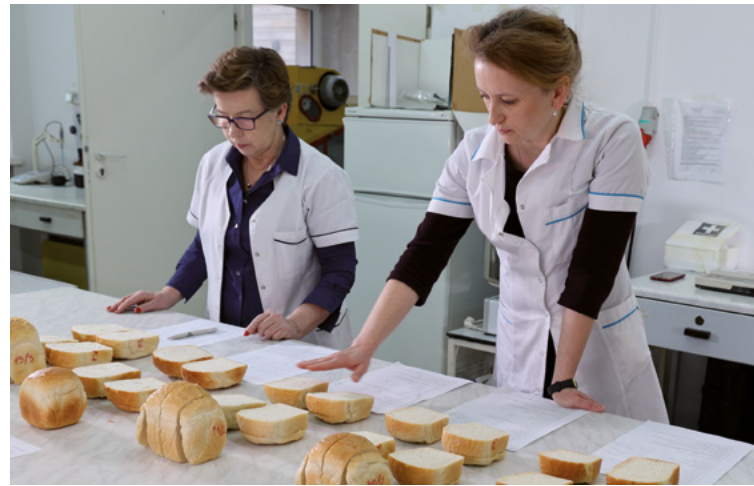
The process of evaluating baked breads from different types of flour obtained in a laboratory baking test
